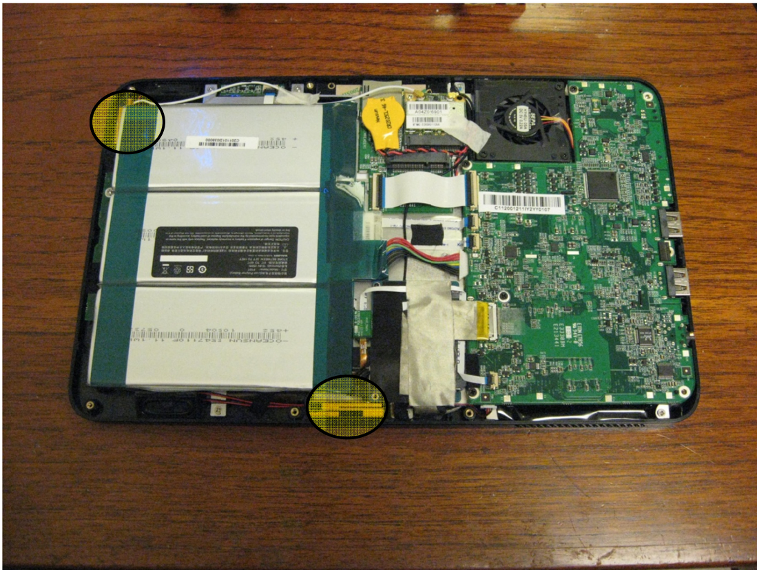
Figure 1 ViewSonic ViewPad 10 Tablet opened to locate the Wi-Fi antennas
